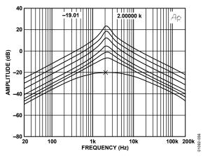
Figure 57. Programmed Amplitude Band-Pass Response
