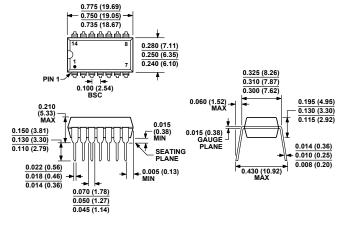
COMPLIANT TO JEDEC STANDARDS MS-001-AA CONTROLLING DIMENSIONS ARE IN INCHES; MILLIMETER DIMENSIONS (IN PARENTHESES) ARE ROUNDED-OFF INCH EQUIVALENTS FOR REFERENCE ONLY AND ARE NOT APPROPRIATE FOR USE IN DESIGN. CORNER LEADS MAY BE CONFIGURED AS WHOLE OR HALF LEADS.
