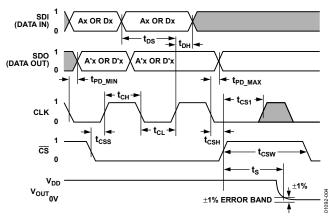
Figure 4. Detailed Timing Diagram
