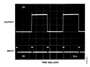
Figure 22. Large Signal Settling Time
