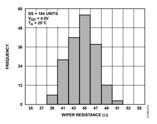
Figure 14. 50 kΩ Wiper-Contact-Resistance Histogram
