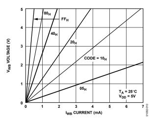
Figure 10. Resistance Linearity vs. Conduction Current
