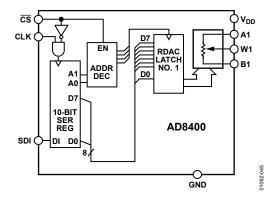
Figure 46. AD8400 Block Diagram
