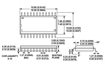
COMPLIANT TO JEDEC STANDARDS MS-013-AD CONTROLLING DIMENSIONS ARE IN MILLIMETERS; INCH DIMENSIONS (IN PARENTHESES) ARE ROUNDEO-OFF MILLIMETER EQUIVALENTS FOR REFERENCE ONLY AND ARE NOT APPROPRIATE FOR USE IN DESIGN
