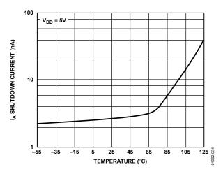
Figure 34. Shutdown Current vs. Temperature
