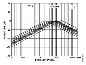
Figure 56. Programmed Center Frequency Band-Pass Response
