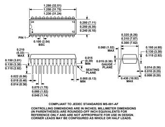
Figure 62. 24-Lead Plastic Dual-In-Line Package [PDIP] Narrow Body (N-24-1) Dimensions shown in inches and (millimeters)
