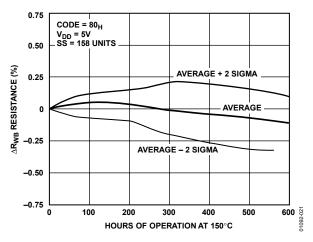
Figure 21. Long-Term Drift Accelerated by Burn-In
