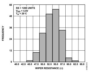
Figure 12. 10 kΩ Wiper-Contact-Resistance Histogram
