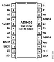
Figure 8. AD8403 Pin Configuration
