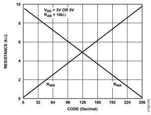
Figure 9. Wiper to End Terminal Resistance vs. Code
