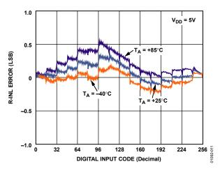
Figure 11. Resistance Step Position Nonlinearity Error vs. Code
