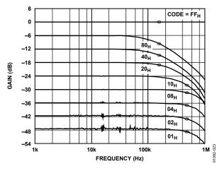
Figure 23. 50 k $\Omega$  Gain vs. Frequency vs. Code
