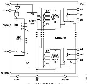
Figure 48. AD8403 Block Diagram
