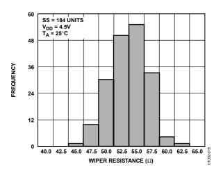
Figure 15. 100 k $\Omega$  Wiper-Contact-Resistance Histogram
