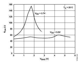
Figure 32. AD8403 Incremental Wiper On Resistance vs. V<sub>DD</sub> (See Figure 39)
