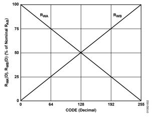
Figure 2. R<sub>WA</sub> and R<sub>WB</sub> vs. Code
