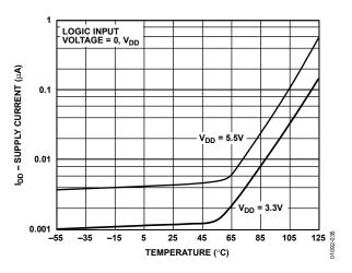
Figure 35. Supply Current vs. Temperature
