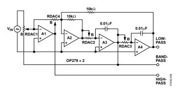
Figure 55. Programmable State Variable Active Filter
