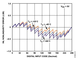
Figure 13. Potentiometer Divider Nonlinearity Error vs. Code
