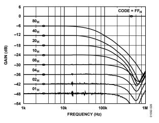
Figure 26. 100 k $\Omega$  Gain vs. Frequency vs. Code
