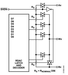
Figure 45. AD8402/AD8403 Equivalent VR (RDAC) Circuit
