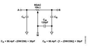
Figure 53. RDAC Circuit Simulation Model for RDAC =  $10 \text{ k}\Omega$
