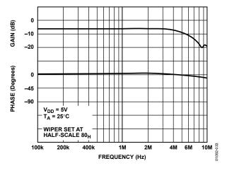
Figure 33. 1 k $\Omega$  Gain and Phase vs. Frequency
