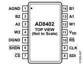
Figure 7. AD8402 Pin Configuration
