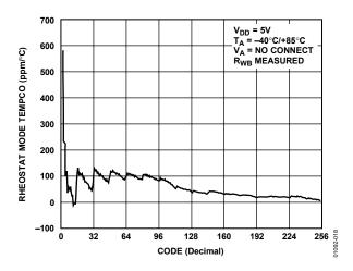
Figure 18.  $\Delta R_{WB}/\Delta T$  Rheostat Mode Tempco
