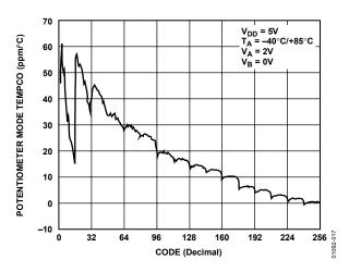
Figure 17. ΔV<sub>WB</sub>/ΔT Potentiometer Mode Tempco
