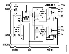
Figure 47. AD8402 Block Diagram
