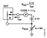
Figure 44. Incremental On Resistance
